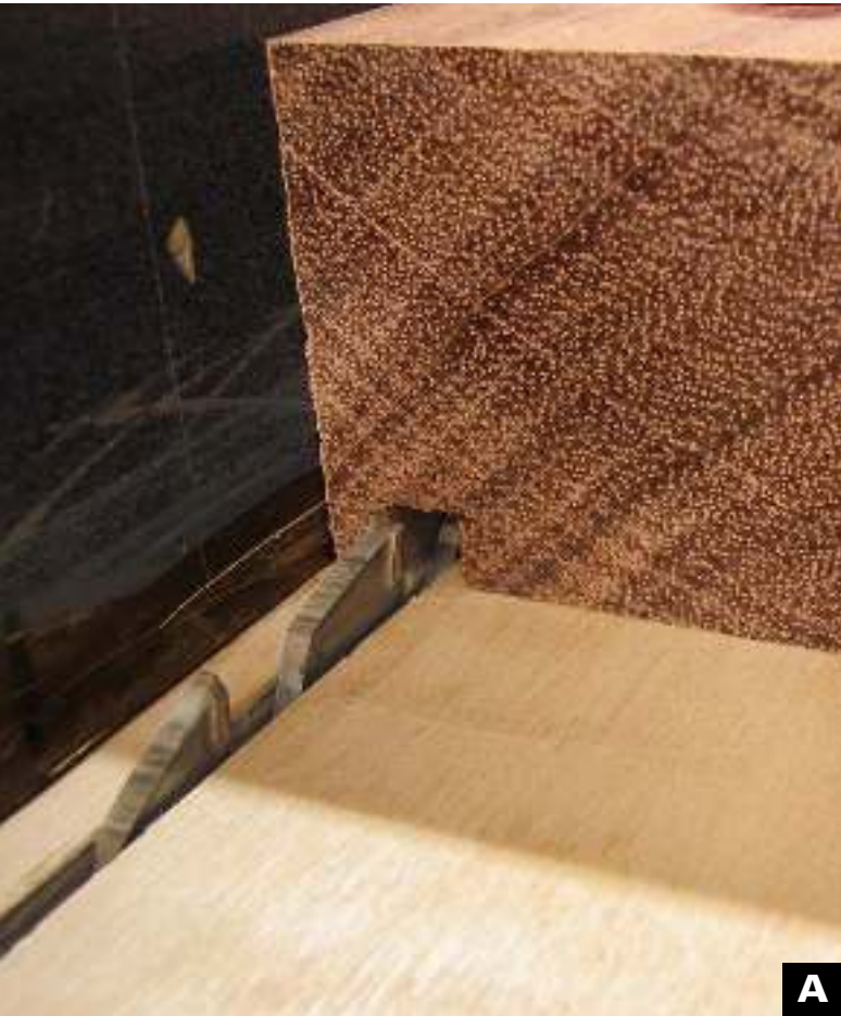
CUT A 1/4-IN. by 1/4-in. groove for the plywood bottom into the four hardwood box parts.
