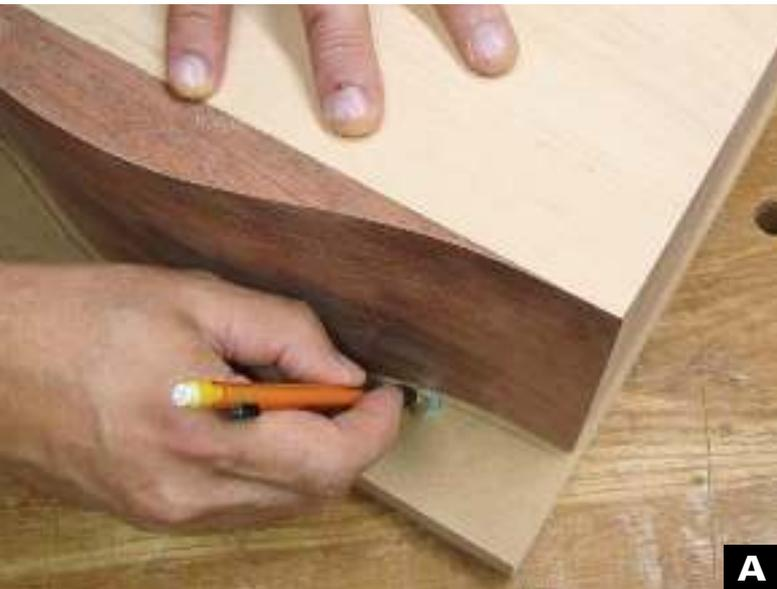
**TO DRAW THE PROFILE** on the MDF clamping caul, place the box on top of the caul and use a pencil and steel washer to draw a line  $\frac{1}{8}$  in. from the front edge of the box front.
