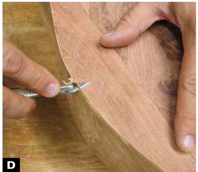
**D** **TRIM THE VENEER** flush to the box using a scalpel. Keep the blade flat to the box and cut slightly inward toward the box to avoid any chipping.
