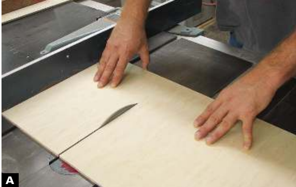
CUT THE BOX TOP and bottom from ½-in.-thick maple plywood.
