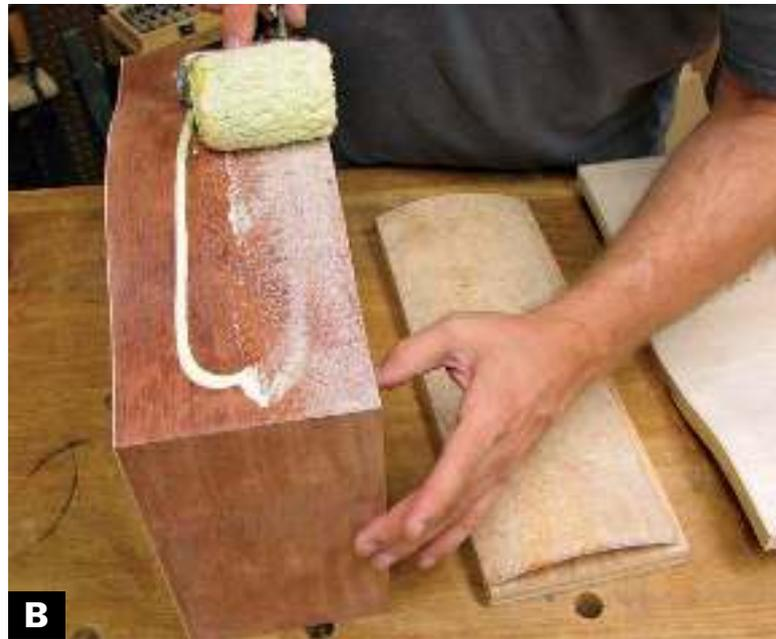
**APPLY A BEAD OF YELLOW GLUE** onto both surfaces; spread evenly with a small paint roller.
