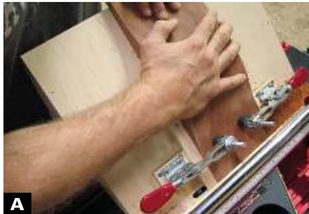
**WITH THE SLED TIGHT** against the router-table fence, push the sled across the dovetail bit to rout the corner dovetails.
