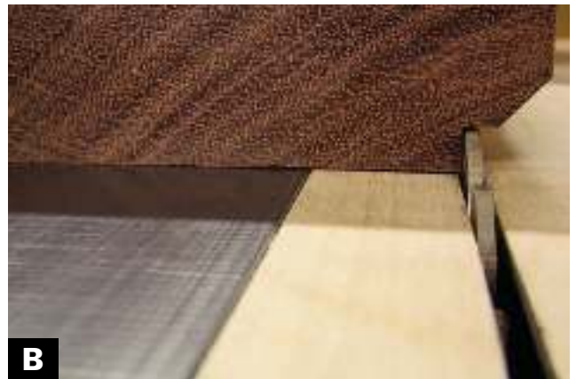
B CUT \frac{3}{16} -IN.-DEEP by \frac{5}{16} -in.-wide rabbets into the front, back, and ends.
