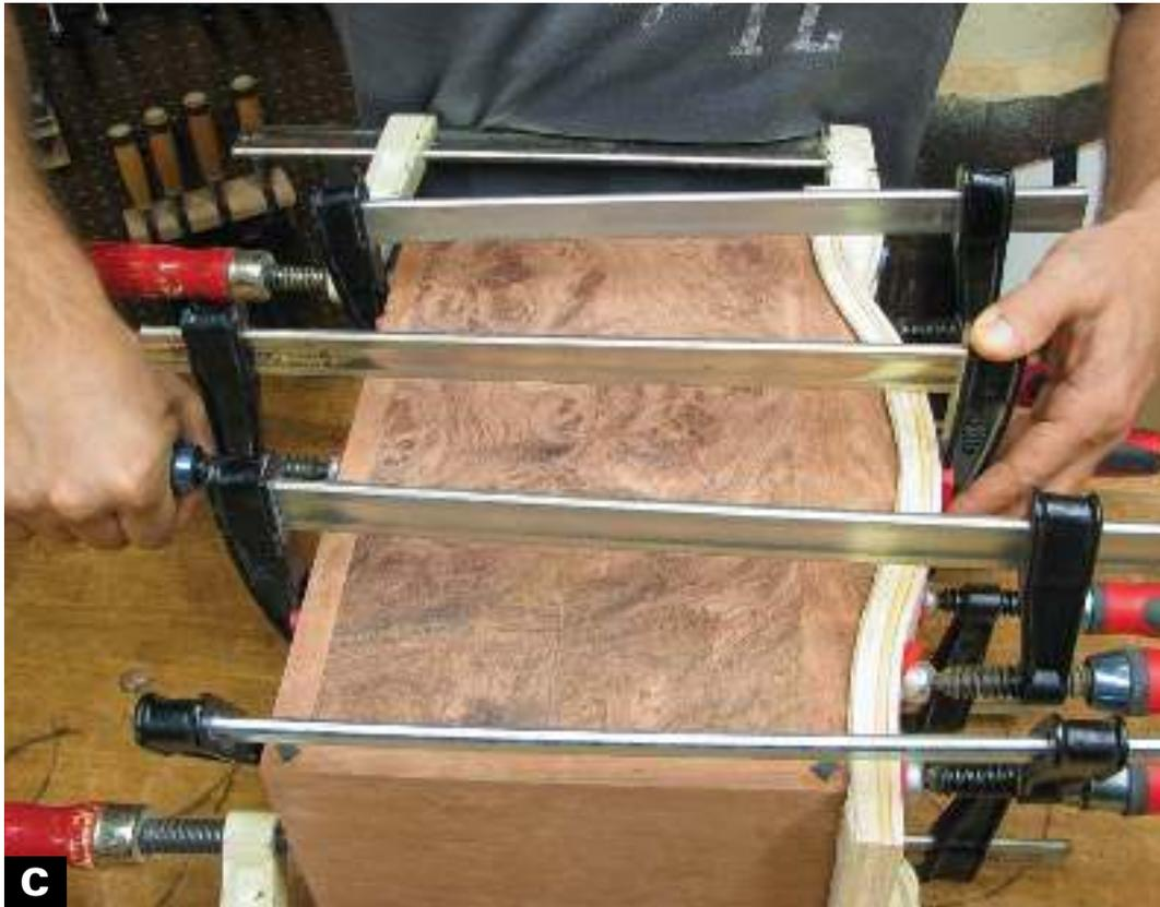
**C** **CLAMP THE VENEER** to the serpentine front with the foam-lined serpentine clamping caul, starting in the middle and working out toward the ends. I suggest using 10 small bar clamps, 5 along each of the lower and upper edges of the box front.
