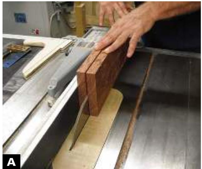
**RESAW THE BUBINGA BLANK** to cut the parts for the box back and ends. Make the first pass with the blade raised to 2 5/8 in. and then flip the blank end for end to make the second pass.
