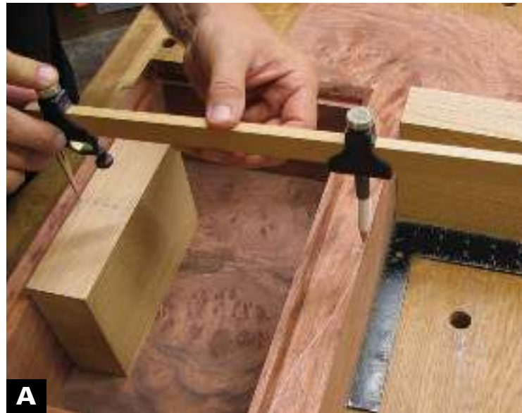
A USE A TEMPORARY BLOCK and a trammel to strike the curved serpentine arc on the box front.
