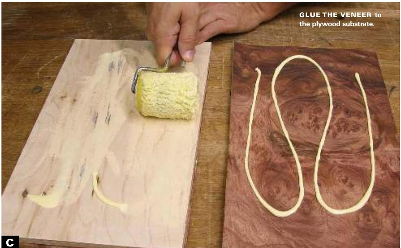
**GLUE THE VENEER** to the plywood substrate.
