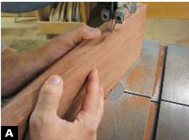
PUSH THE BOX FRONT through the blade at a steady pace with even pressure to avoid an uneven sawkerf.
