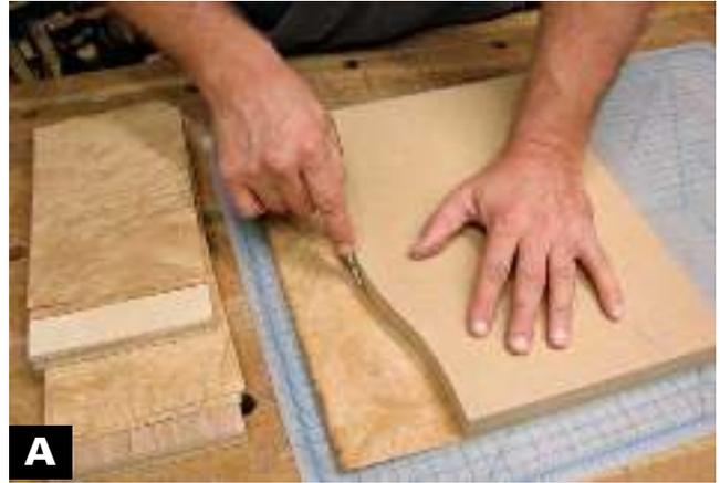
**CUT THE VENEER** by pressing down firmly with one hand and using a scalpel to cut along the caul.
