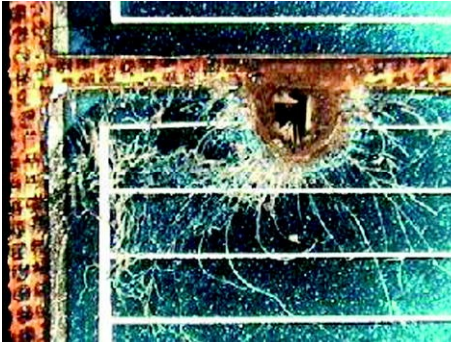
Fig. 1.1 Puncture in Hubble Space Telescope array cause by space debris (Image courtesy of NASA)
