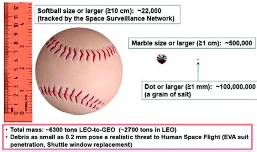
Fig. 1.3 Breakdown of the 6,300 tons of mass in Earth orbit (Graphic courtesy of NASA.)
