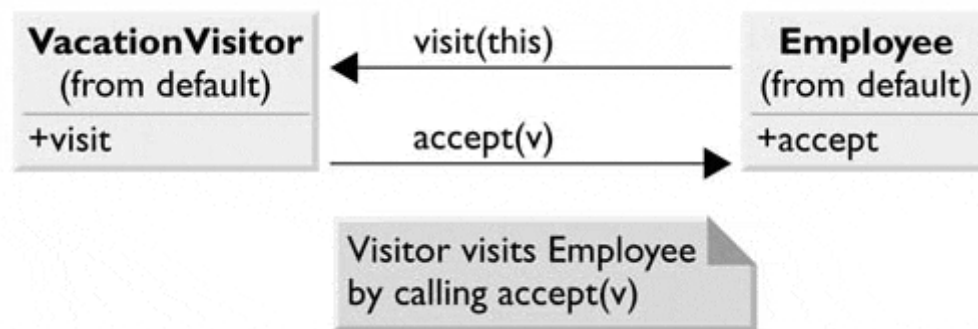
Figure 2.7. A comment is often shown in a box with a turned-down corner.
