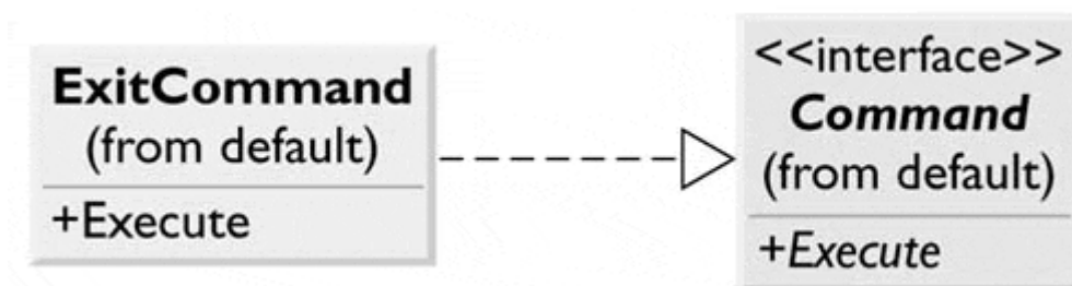
Figure 2.4. ExitCommand implements the Command interface.
