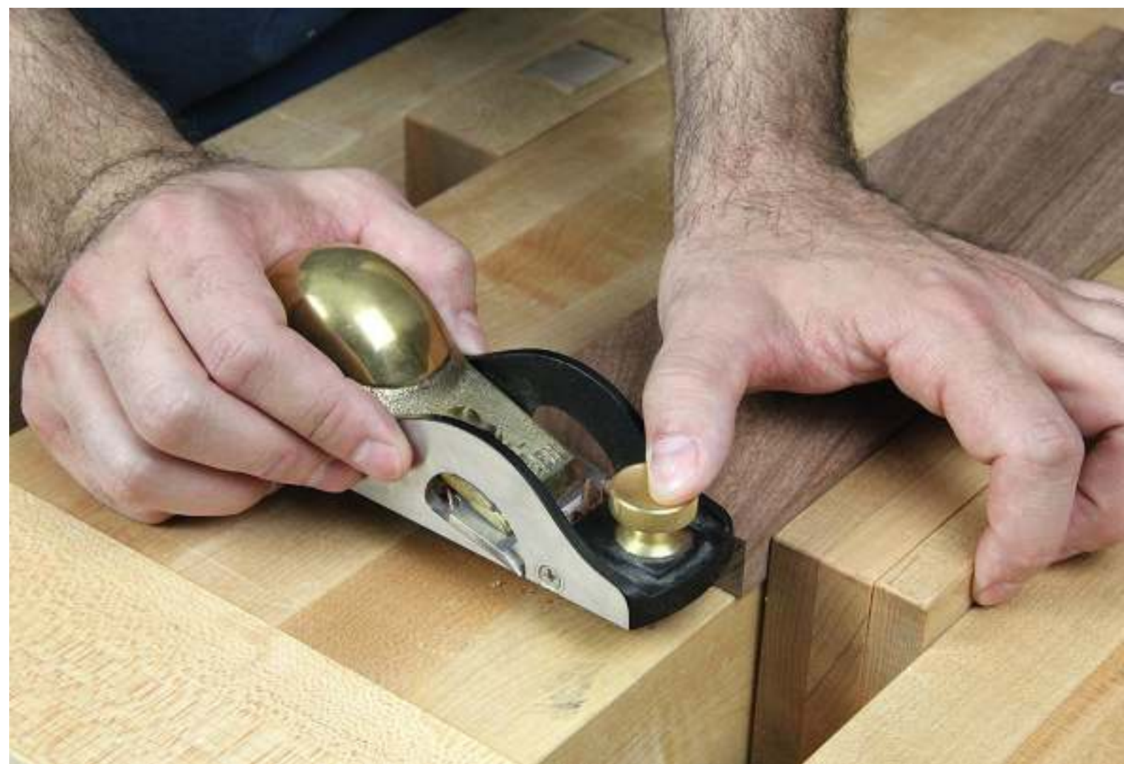
Clean Your Cheeks A rabbeting block plane excels at cleaning up the cheeks of a tenon.
