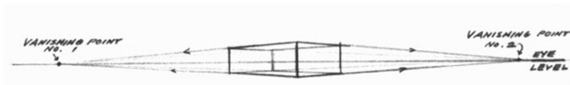
**Figure A.** At eye level the converging lines of the sides of the box come down from the top edges and go up from the bottom edges to meet and vanish at imaginary points on the horizon (or eye level) called vanishing points.
