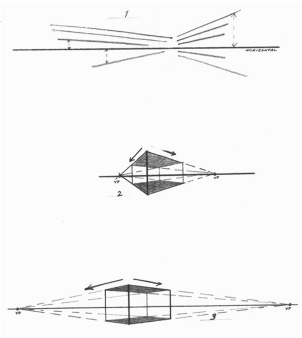
**Figure G.** Ask yourself how much the line of an object departs—up or down—from the horizontal, as the diagram shows at view 1. If the diagonals are incorrect, you get the distortion shown at view 2. Note that the proper angle at view 3 gives you the correct form, because the diagonals run farther out to their vanishing points.
