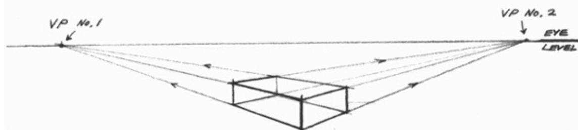
**Figure B.** When the cubic object is below eye level, all converging lines go up to their respective vanishing points. The arrows show the direction in which the parallel lines extend to the eye level.
