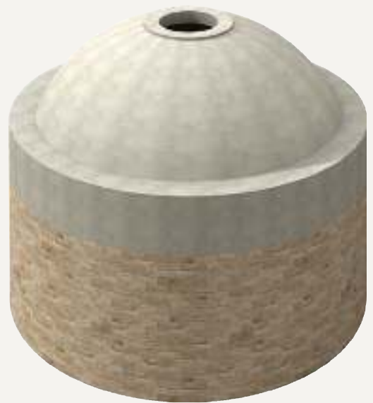
Hemispherical dome with oculus
