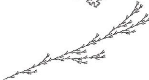
4. A squig curve (above) and a fractal grass (below) with their generators: the line segments in the generators are repeatedly replaced by scaled down copies to form the fractals
