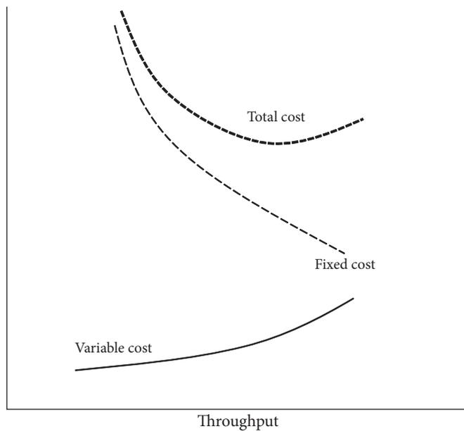
FIGURE 2.1 *Transportation costs as a factor of pipeline diameter*
