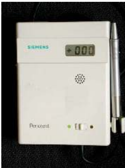
Figure 2-15 Periotest™ device for the objective evaluation of tooth mobility.
