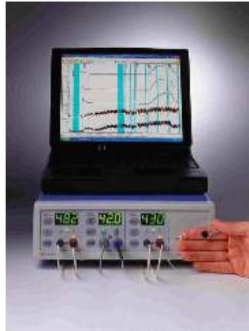
Figure 2-16 Laser Doppler flowmetry device for the possible detection of pulpal blood flow and vitality.
